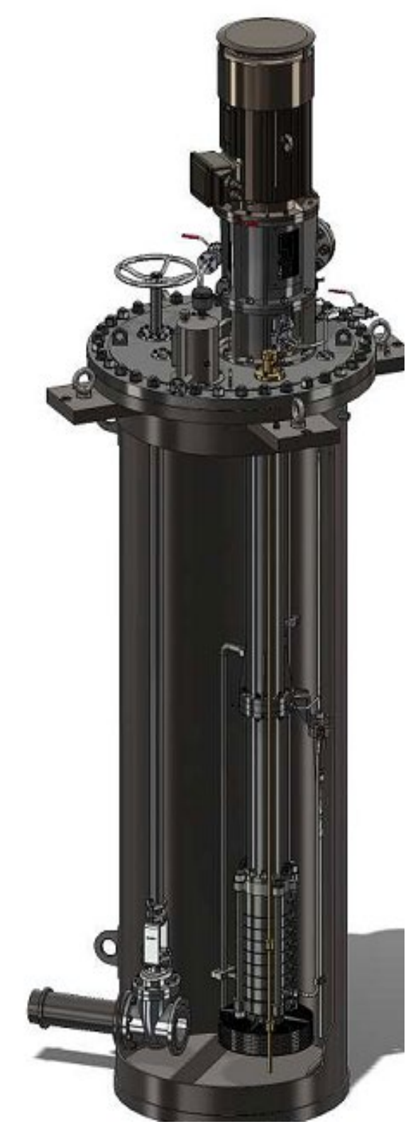
Oil Leakages Dain Pumps Models: NOU (НОУ); NV (НВ) Flow range: 10-70m 3 /hr; Head range: 50-900m.
